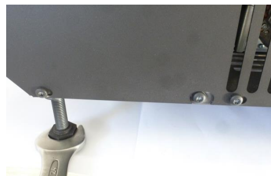
Figure No.4 - Close up of the 24 mm wrench for adjusting the legs
